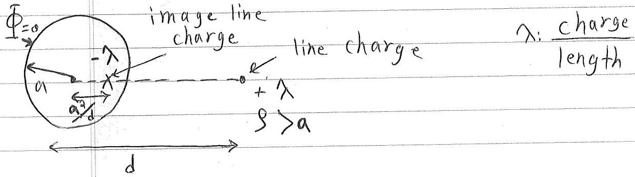
The image line charge gives rise to the same boundary condition,  $\Phi = \Phi_0$  on the surface of the cylinder and exactly the same potential outside the cylinder ( $r > a$ ).
