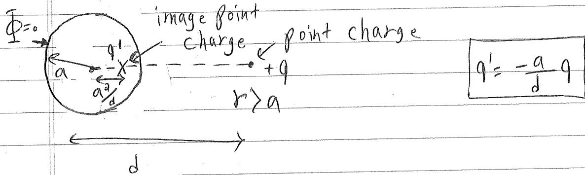
The image charge in this case is a point charge  $q' = -\frac{a^2}{d} q$  situated at a distance  $\frac{a^2}{d}$  from the center of the sphere.
