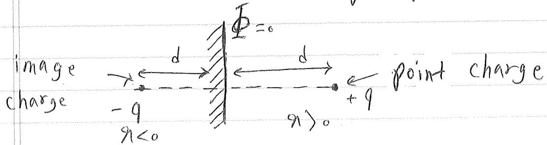
For a charge  $+q$  in the region  $\mathbf{r} > 0$ , with  $\Phi = 0$  at  $\mathbf{r} = \mathbf{a}$  we can use a point charge  $-q$  in the region  $\mathbf{r} < 0$  located at the image of the given charge. This gives rise to the same boundary condition, and hence the same potential everywhere at  $\mathbf{r} > 0$  by the uniqueness of solution for a Dirichlet problem.
